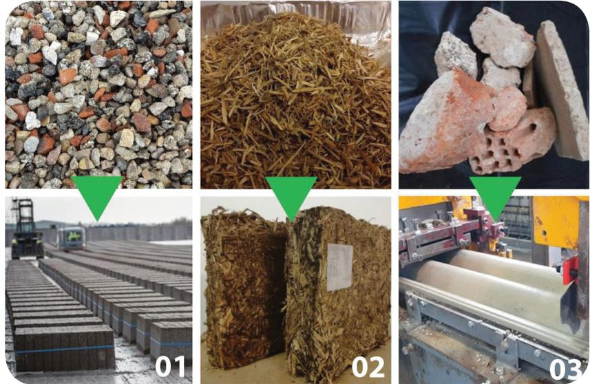
Examples of the RE<sup>4</sup> components: 01 – Concrete building blocks made of CDW mineral aggregate; 02 – Insulation panels made of CDW wood fibers; 03 – Reconstituted roof tiles made of CDW bricks and tiles
