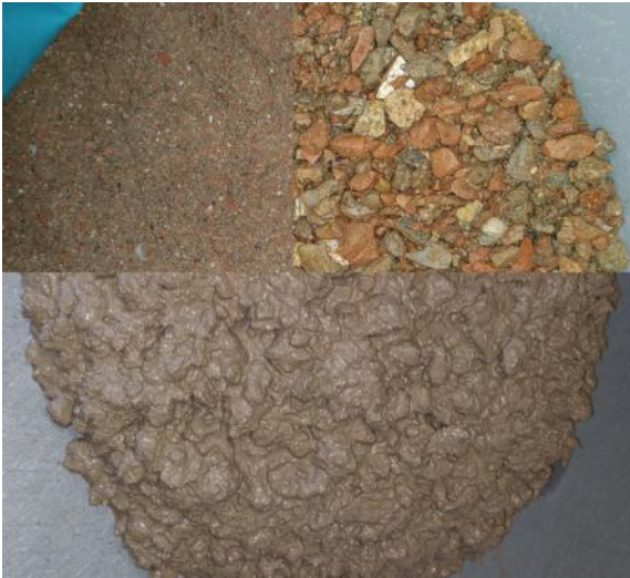
Figure 4: Concrete mix with mineral CDW aggregates for precast stone production
