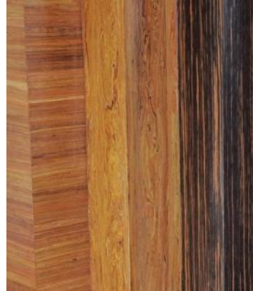
Figure 29: Songwood, compressed wood composite from recycled timber for internal partition wall application, Source: www.architectmagazine.com
