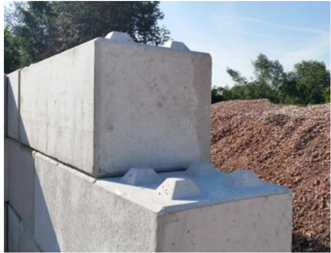
Figure 5: Precast concrete stones made from mineral CDW aggregates
