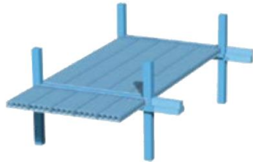
Figure 12: Hollow-core slab elements on inverse T-beams on multi-storey columns
