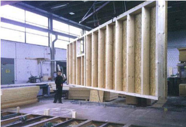
Figure 34: Prefabrication of timber frame elements in the workshop, Source: Benedikt Wagner, Holzbau Schenk GmbH
