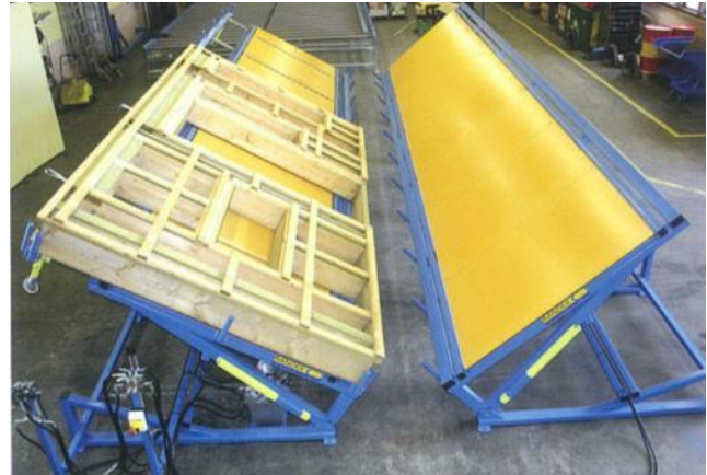
Figure 35: Turning table for easy assembly of timber frame in the workshop, Source: Randek AB
