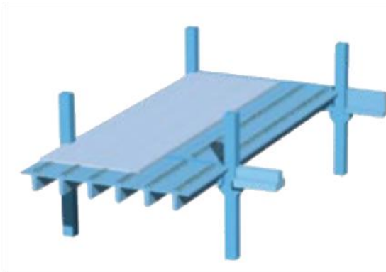
Figure 11: Semi-precast TT-slab elements on inverse T-beams on multi-storey columns
