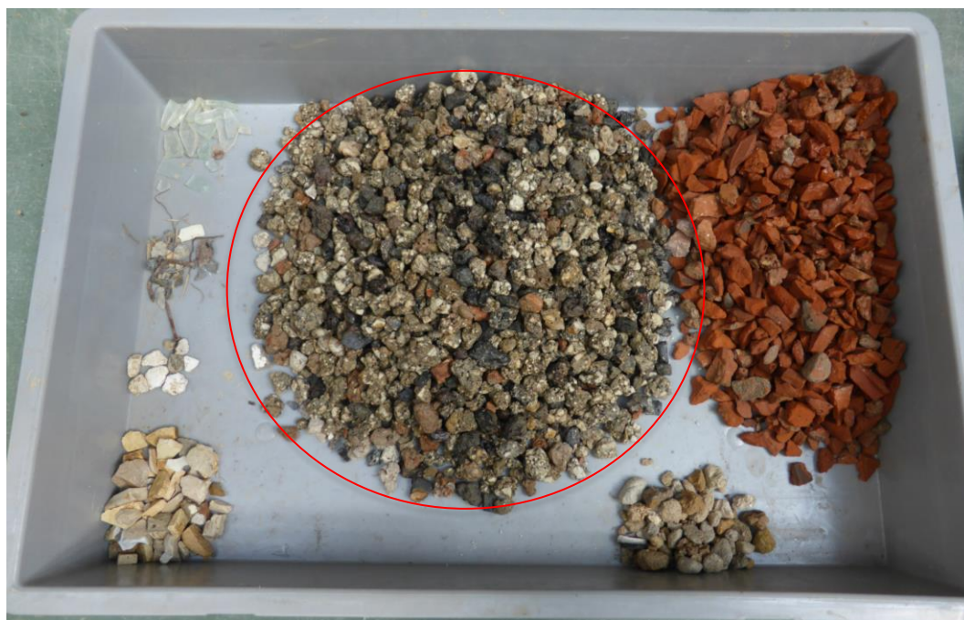
Figure 1: Improved sorted CDW of size-fraction 8/16 mm (pile marked with red circle), surrounded by components that have been sorted out. Upper image is from Northern Europe (NE B1), lower image from Southern Europe (SE B1).
