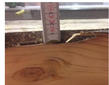
Figure 3. Strength grading: assessment of defects, decays, cracks and dimensions, location + orientation of branches
