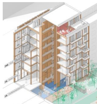
Figure 23. Skeleton system with stiffening core
