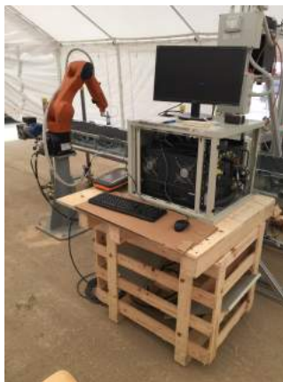
Mobile CDW robotic sorting system
