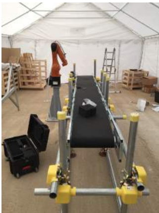
Mobile CDW robotic sorting system
