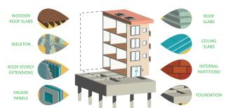
Up to 80-90% of reusable structures for RE<sup>4</sup>-prefabricated building concept
