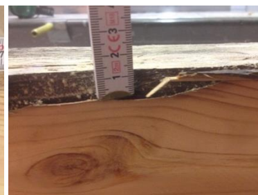
Figure 5. Strength grading: assessment of lamellas regarding dimension, location and orientation of branches, defects, decays and cracks.
