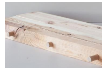
Figure 13. Small scale ceiling sample with dowels
