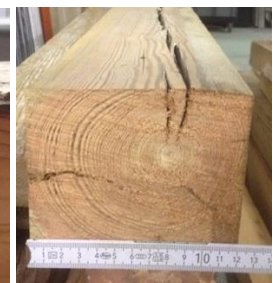
Figure 5. Strength grading: assessment of lamellas regarding dimension, location and orientation of branches, defects, decays and cracks.
