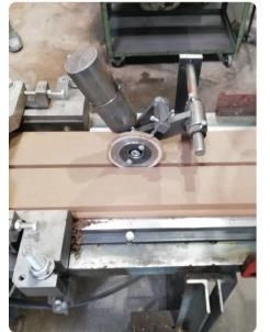
Longitudinal cutting phase of *Marmoroc type RE<sup>4</sup> extruded tiles*
