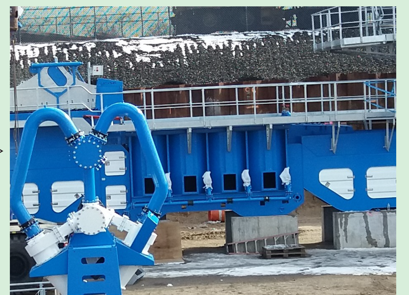
Set of 4 attrition cells incorporated into a C&D plant in New York, USA
